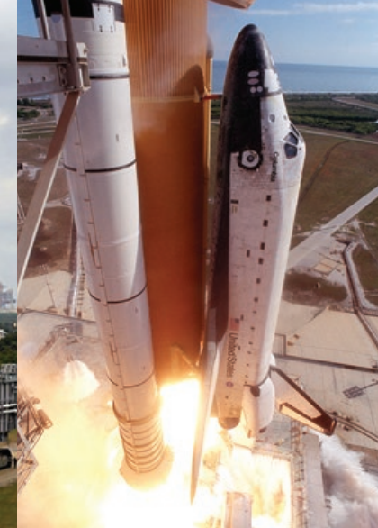
Columbia lifting off on her final mission. The small, light-colored triangle visible at the base of the strut near the nose of the orbiter is the Left Bipod Foam Ramp.
