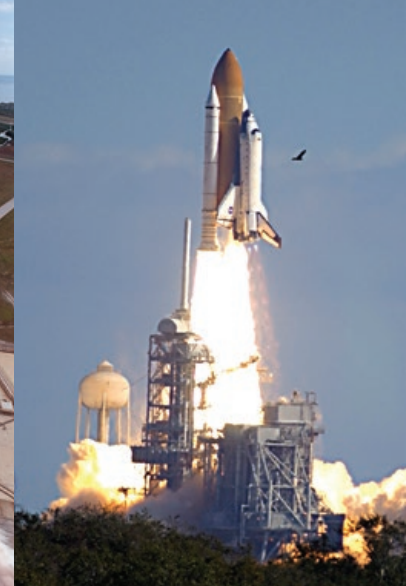
Columbia lifting off on her final mission. The small, light-colored triangle visible at the base of the strut near the nose of the orbiter is the Left Bipod Foam Ramp.
